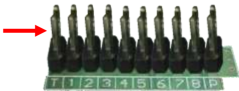
Abb. 3 Jumperblock; T= Position Abschluss-Widerstand, P = Parkposition für Reservejumper
